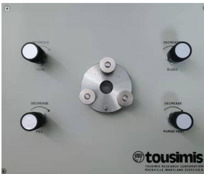
Control board. The chamber is in the center.
