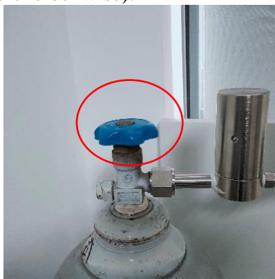
CO 2 tank valve
