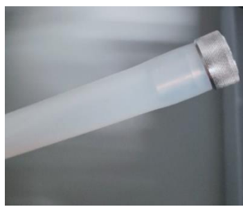
Drain tube closed with a metal plug
