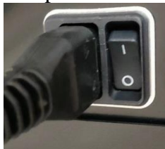
Main Switch(Off Position)
