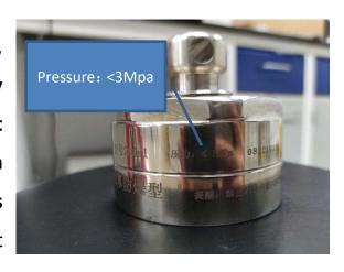
use the equipment in normal operation, it is **strictly forbidden to operate with pressure**, which not only damages the equipment, but also has safety
