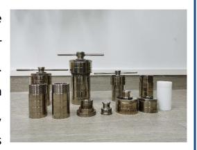
a common small reactor for scientific research in university teaching and research units. In the laboratory, we usually use the hydrothermal kettle,
