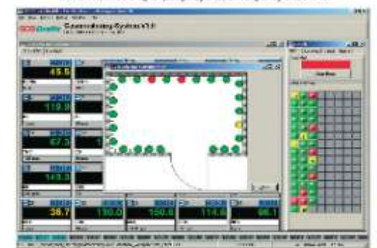
GasCom, graphic display of cylinder pressure with alarm functions and low supply pressure displays
