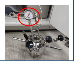
Mpa gauge, pa gauge, 10Mpa gauge and so on. When performing pressurized reaction, you must make sure to check the unit of measurement of the pressure gauge which is in on range of the reaction!
