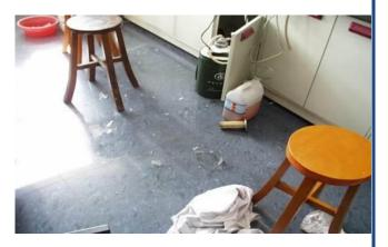
160°C. While the person was observing the temperature of the oil bath, the sealing tube suddenly exploded and the whole reaction system was completely blown apart. The person was injured on the forehead and was lucky to be wearing eye protection at the time so that both eyes were not harmed
