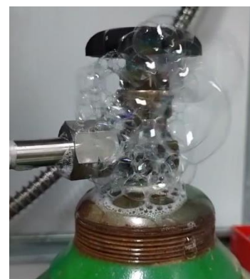
Figure 1 Heavy leakage from the bottle top
