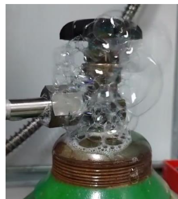
Figure 1 瓶口泄露严重
